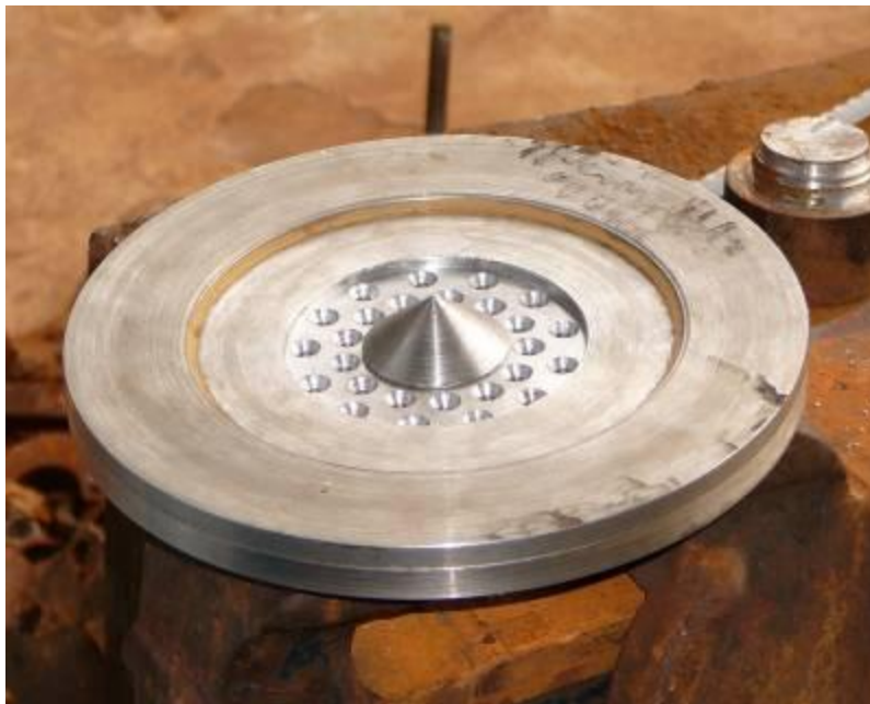
A new plate with centre cone and conical inlets to holes. Number of holes reduced from more than 100 to 27. There are only holes where material is moving inside the extruder.
