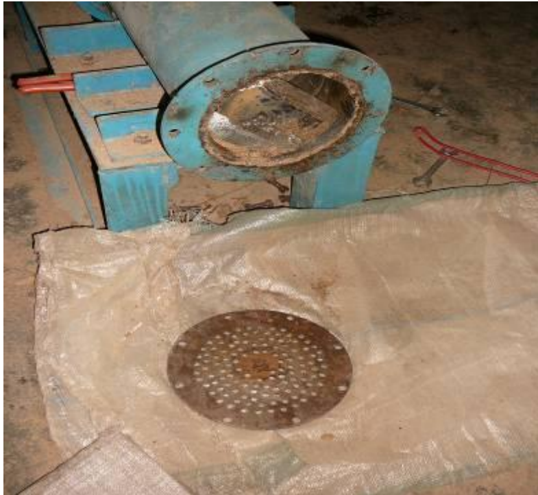
A typical die plate, flat with a maximum of straight and rough holes.
