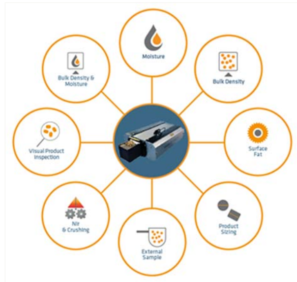
Figure 1. Inline sampler with option for multiple analytical sensors to be integrated
