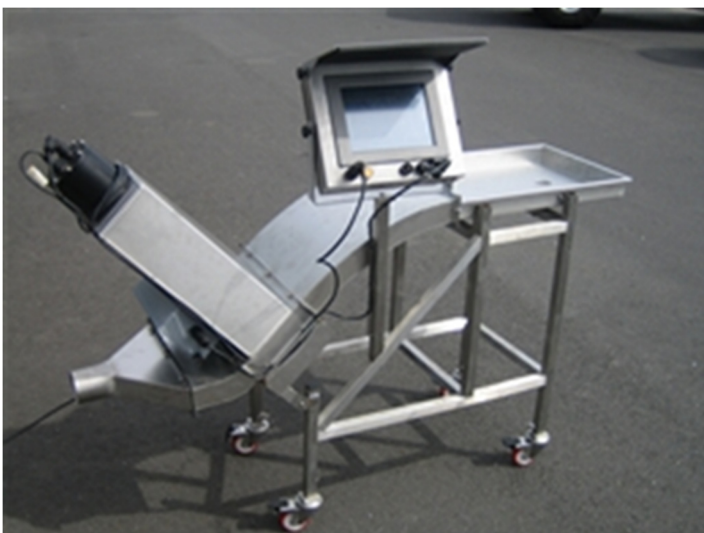
The iScan IM system: online image process analysis of pellets. Weighing, size and color measurement.
