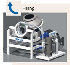
The drum is filled with the product to be processed. Weighing and proportioning are carried out by high -precision load cells integrated in the vacuum coater. The drum swings into working position and rotates.
