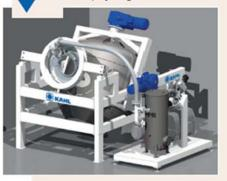
The drum is emptied by a pivoting movement downwards. Meanwhile, the drum continues to rotate. Complete emptying is ensured.
