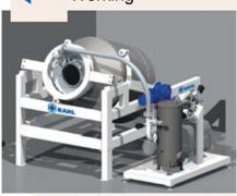
In the working position, the vacuum is generated and then one or more liquids are sprayed, one after the other, onto the product. (Nozzles and liquid addition are not shown). The vacuum is broken in a defined way.
